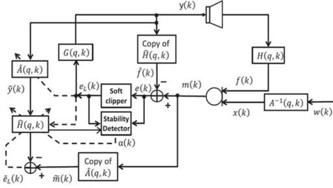
Fig. 1. Block diagram of the used AFC scheme
