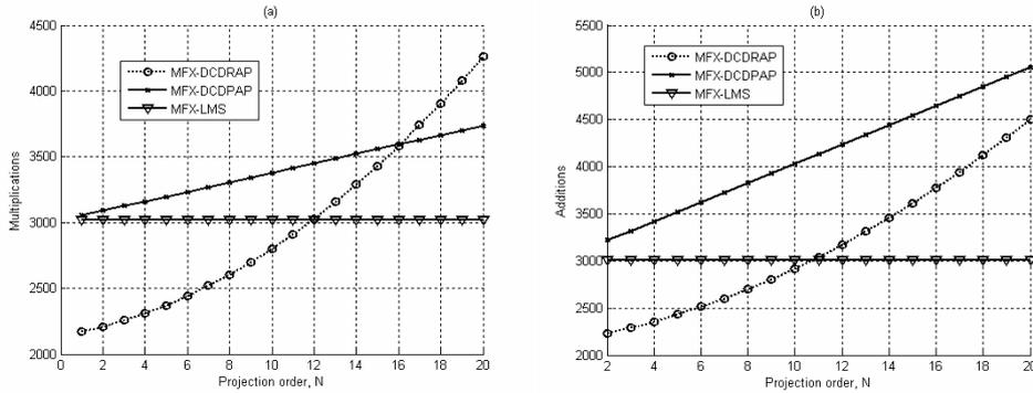
Fig. 2 – Numerical complexity of the MFX-LMS, MFX-DCDRAP and MFX-DCDPAP algorithms ( $I = 1, J = 3, K = 2, L = 150, M = 64, N_u = 4, M_b = 16$ , and  $N$  is varying); a) number of multiplications per algorithm iteration; b) number of additions per algorithm iteration.
