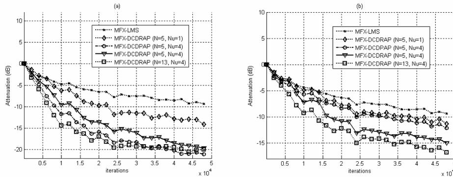
Fig. 3 – Convergence curves for multichannel delay-compensated modified filtered-x algorithms for ANC with ideal plant models ( $I = 1, J = 3, K = 2, L = 150, M = 64, M_b = 16$ ); a) ideal plant models; b) noisy plant models (10 dB SNR).
