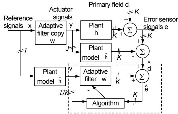
Fig. 1 – A delay compensated or modified filtered-x structure for active noise control [2, 4].
